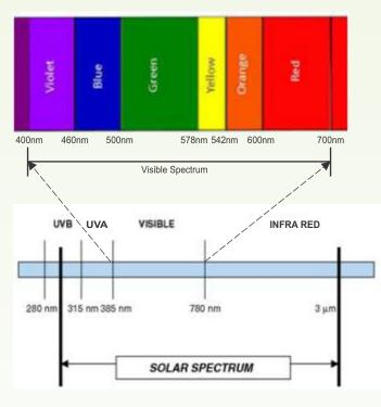
5% of the total solar energy reaching the earth is UV light. This part of the solar spectrum leads to degradation / weathering of polymers by breaking chemical bonds.
