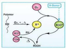
The schematic shows the degradation of polymer (RH) by heat ( $\Delta$ ), light ( $\tau$ ) & oxygen(O2). The reaction is sustainable as free radicals (R\*, ROO\*, RO\* & OH\*) are continuously produced by polymer degradation.
